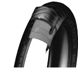
BELTED TYRE WITH RADIAL CARCASS (90 DEGREES)
